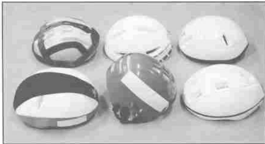
Figure 3. The six types of bicycle helmets used in this series of tests include left to right: In the top row no-shell with attached external rubber straps; hard shell; micro-shell. Bottom row: no-shell with removable nylon cover, hard shell with increased occipital coverage; micro-shell with embedded liner net.
