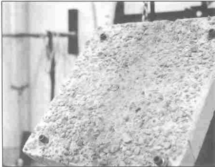
Figure 2: Rough concrete slab with small pebbles embedded into the surface (see penny for size comparison to pebbles).
